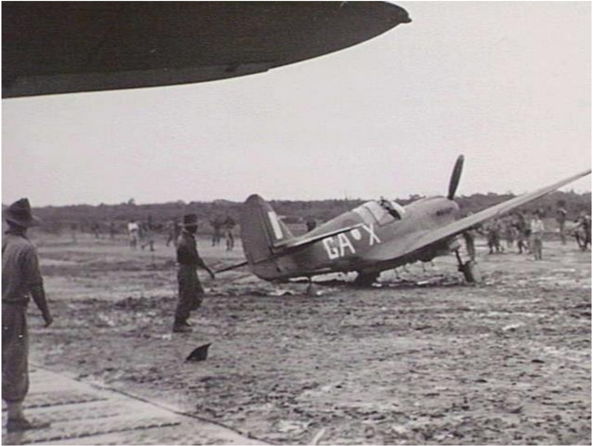
75SQN Kittyhawk damaged after landing on the soft and boggy Tarakan Airstrip, highlighting the challenges faced by the squadron and its personnel in the first month after landing on Tarakan on 1 May 1945. (AWM)
